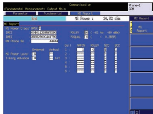
Mobile Terminal Report Monitor (GSM)
